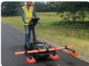
← 3 sensors offer a wider range of measurements for entire pavement and joint coverage
